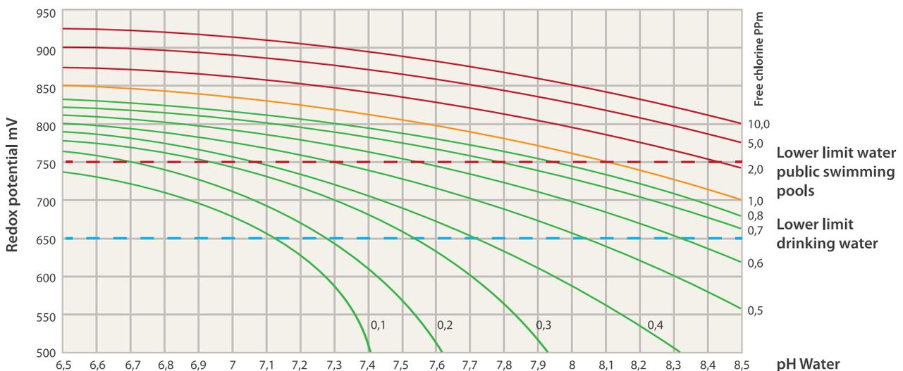
A simple method for ascertaining whether particular water is compatible with the use of PP pipes is to measure the oxidation-reduction potential using one of the many portable instruments available on the market, such as the one shown in the picture on the top. The potential must be less than 750 mV
