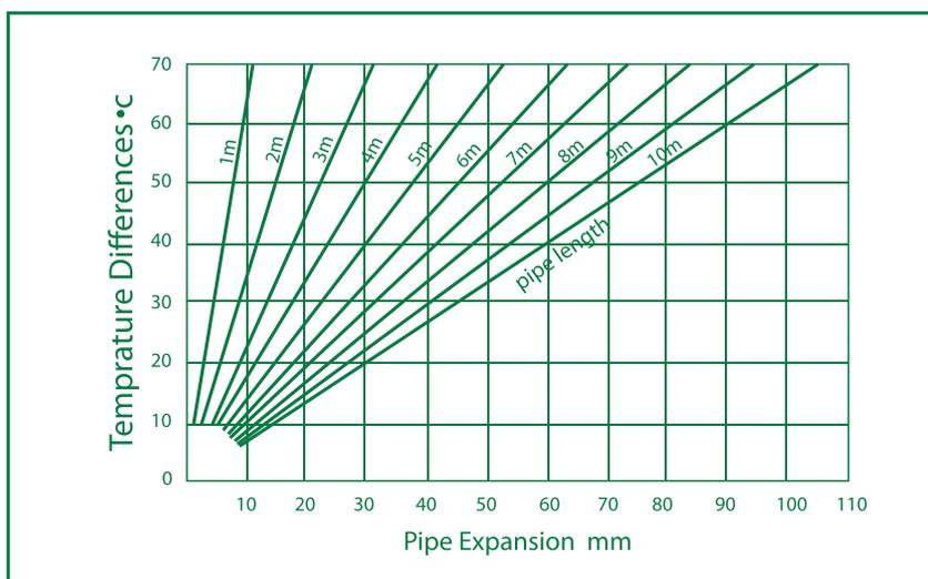
Changes in the length of a pipe regardless of its diameter and thickness is calculated by the following formula:
