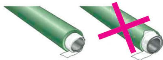
**Connection between fittings in PP-R and iron pipes**
