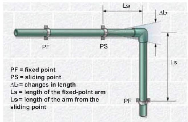
Once the length of the section is known  $L$ , the elongation  $\Delta L$  is determined using the formula:
